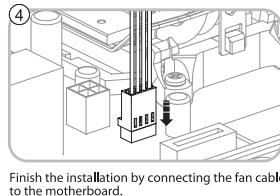
Finish the installation by connecting the fan cable to the motherboard.
