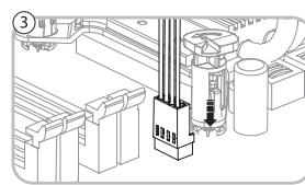
Finish the installation by connecting the fan cable to the motherboard.
