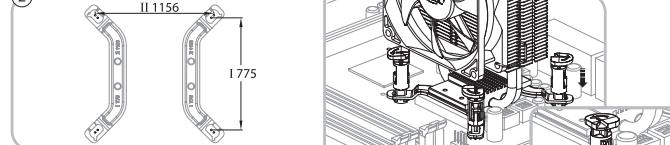
Put the cooler on the processor, check your socket type and ensure all push-pins through the motherboard mounting holes. Position the clip as shown in the picture and then push down to secure the cooler.
