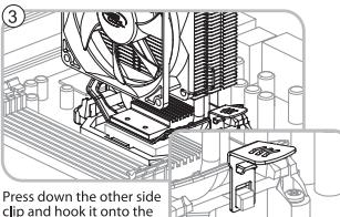
Press down the other side clip and hook it onto the tab, too. Please ensure perfect contact between the heatsink base and the CPU surface during installation.
