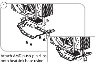
Attach AMD push-pin clips onto heatsink base using the screws.
