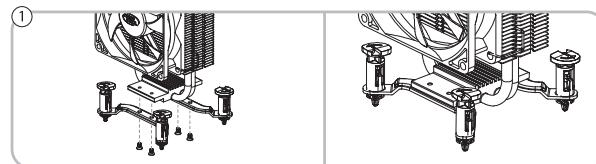
Attach Intel push-pin clips onto heatsink base using the screws.
