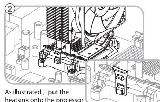
As illustrated, put the heatsink onto the processor and hook the vertical clip onto the retention frame tab.
