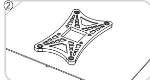
Place the AMD back plate on the back of the motherboard.
