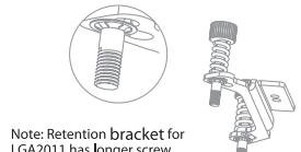
Secure the bracket to heatsink base using the hole C; and position the bracket screws on the hole C too.
